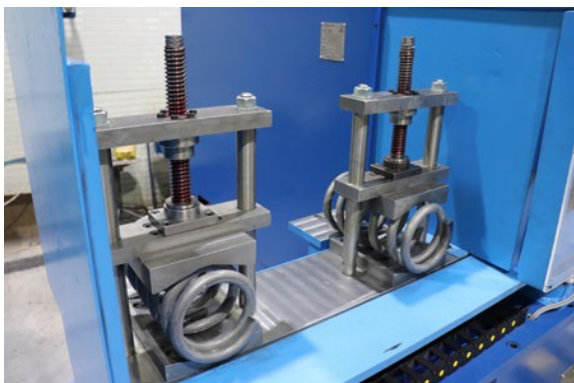
Loading Plate ready for grinding
