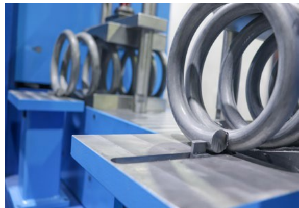
Limiter for setting equal distance of springs from the grinding wheel
